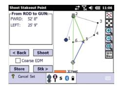
Once you are close to the point, the display changes to a precise position display. It's easy and fast to get the rod right on the point.
