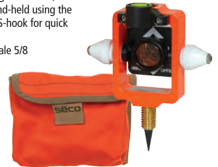
6405-10-FOR — 25 mm Stakeout Prism Assembly
